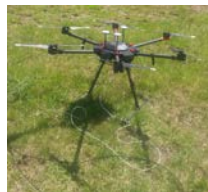
UAV drone used for antenna pattern measurement
