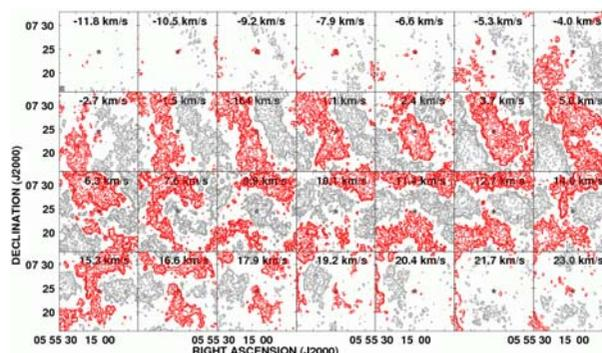
VLA channel maps, all baselines. The positive contours are in red, and the negative ones in grey. The synthesized beam has a size of  $\sim 35$  arcsec.
