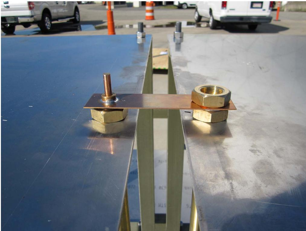
Figure 2. Top cap plate adjusted to 0.61" from panel set to gap of 1.955".
