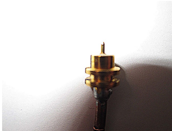
Figure 5. Example of SMA connector with raised dielectric which presents metal-to-metal contact of the outer conductor at the reference plane.
