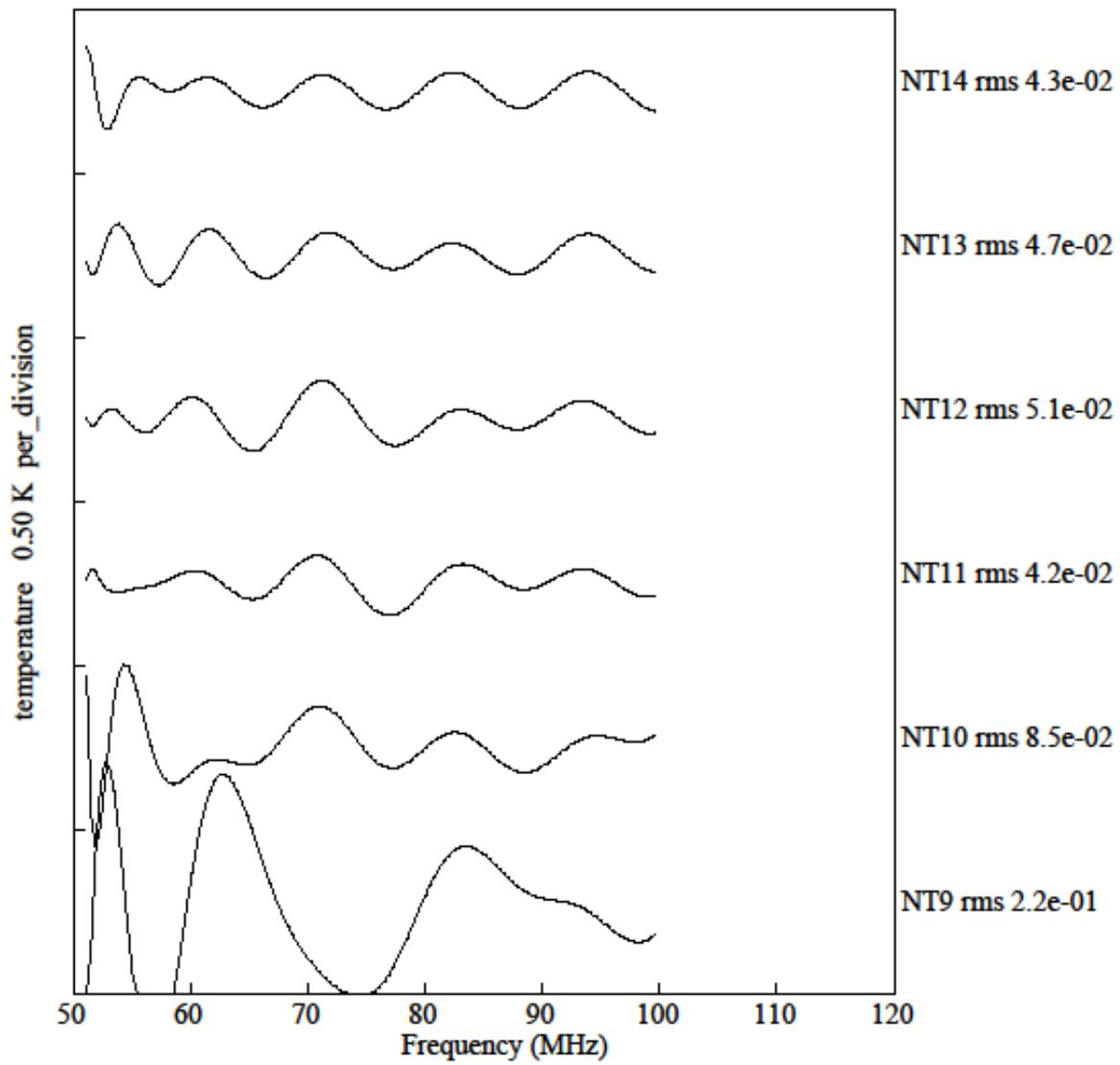
Figure 4. Simulated residuals for lowband2 2020 S11 at GHA = 12 hours vs number of terms in the smoothing filter.
