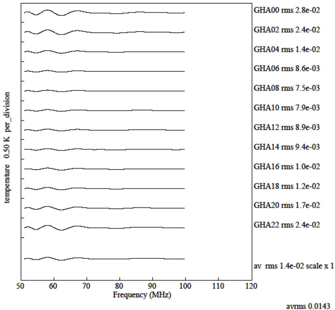
Figure 1. Simulated residuals for lowband 2016/2017 data for a change from a Fourier fit to 12 polynomial terms with 5 physical terms removed
