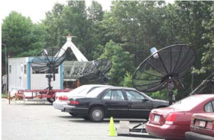
Fig. 1- View of 3 small radio telescopes tracking the Sun in the parking lot of MIT Haystack Observatory at latitude 42.5°N 71.5°W. Observations were taken in “VLBI” mode with 4 MHz bandwidth centered at 1417 MHz. GPS timing was used to synchronize the timing and local oscillators.
