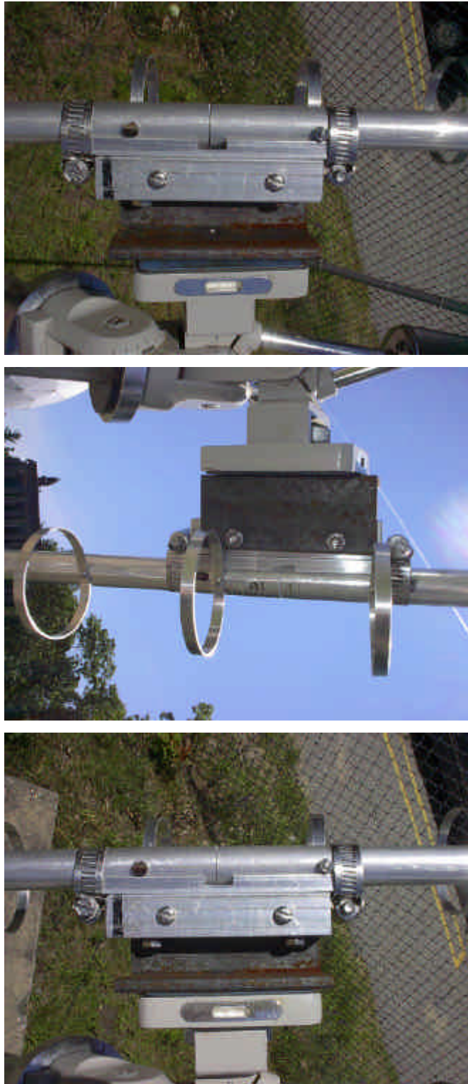
Figure 5.) Yagi mounting configuration to standard camera tripod. The mount was made by taking a piece of steel and threading a hole into the center for the camera screw to attach to. Then identical holes to the ones that come with the Yagi were placed into it to join the mount to the L piece to the Yagi for a strong and easy attachment.
