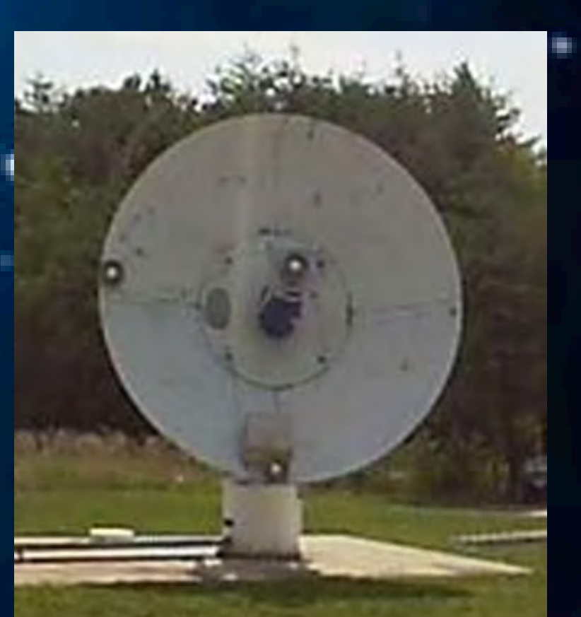
Figure 9: What the dish that took figure 8 image looks like. It has a microwave absorber unit on the bottom, an equipment case cover on center left and the feed structure in the center. 4
