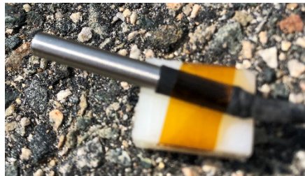
Figure 1: Test probe set up used to measure free air temperature.
