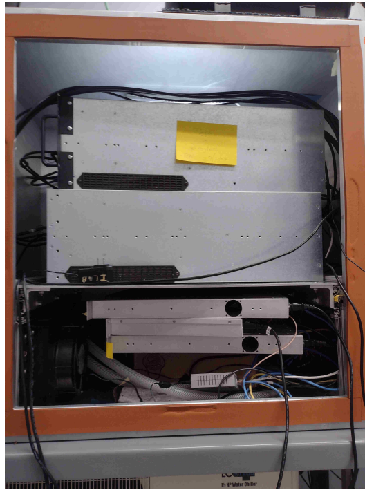
Figure 1: The Mark6 and expansion chassis in the hypobaric chamber. The two R2DBEs and timing distribution box are underneath the support shelf. The RPi SBC is to the left of the R2DBEs, while the black air circulation fans and radiators are visible to the right side. The water circulation hose and 1G network switch are visible just beneath the R2DBEs.
